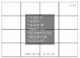
[STATUS] S/W VER: V1.0.10-tv\_16 (06/05/08 10:07) [HDD] A: 150G(63%) B: NONE C: NONE D: NONE MAC: 00.0E.B5.00.06.32 DDNS: SERVER (null) FAIL SIZE 720\*576 [REC] CH RA QUAL CH RA QUAL CH RA QUAL CH RA QUAL 2 BEST 5 2 BEST 9 2 BEST 13 2 BEST 2 BEST 6 2 BEST 10 2 BEST 14 2 BEST 2 BEST 7 2 BEST 11 2 BEST 15 2 BEST 2 BEST 8 2 BEST 12 2 BEST 16 2 BEST Fig3.3.2 Status view
